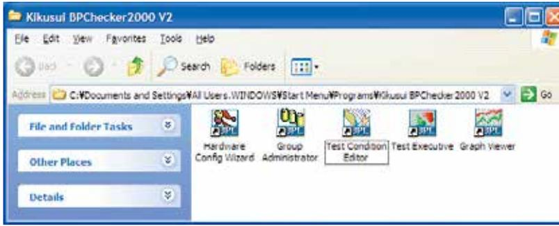
The “BPChecker 2000 Basic Edition”, a standard accessory, can manage the entire operation from the setting of the test conditions, the execution of the test, and analyzing the test result files. This software can control the thermostatic chambers (manufactured by ESPEC) and also applies to the synchronized test with the thermostatic chambers.
