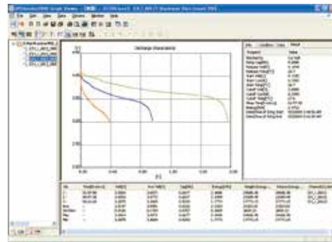
▲ Example of screen display: The charging (discharging, charging + discharging) curve can be overlaid on the display. The average, standard deviation, maximum value and minimum value for the overlaid data can also be calculated for data analysis.
