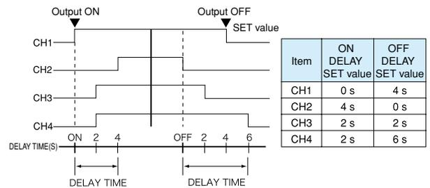
Note: The actual rise time after the output is turned on and the actual fall time after it is turned off differ depending on the output and load conditions. The conceptual drawing ignores the rise and fall times. Also, there is an internal processing time from the time the OUTPUT switch is pressed until the output is turned on or off, so that even if the time is set to 0 s, there will be an error of several tens of milliseconds.
